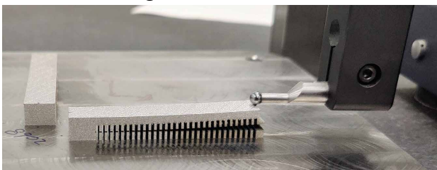
Figure 3. X,Y-beam calibration method provides insight in orthotropic behaviour.
