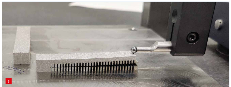
X,Y-beam calibration method provides insight in orthotropic behaviour.
